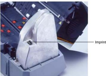
The imprinter connector should be protruding from the opening on top of the circuit board cover.
